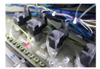
Vacuum transformation of the robot arm for sucking batteries: The original vacuum generator is removed, and the vacuum is directly provided by the factory vacuum pump. Only the solenoid valve is needed to control the on-off of the vacuum source, which can avoid the leakage loss of compressed air and improve production efficiency.
