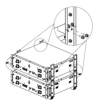
c. A maximum of four battery module are stacked based on the system capacity.
