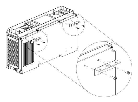
Refer to the following for the recommended the wall mounting assembly (angle bracket + L-bracket) installation:
