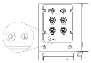
Figure 4-1-1 Schematic diagram of equipment grounding
