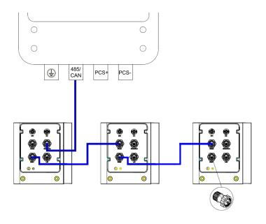
Figure 4-3-2b Communication wiring of multiple system
