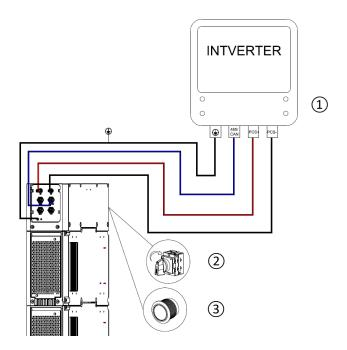
Note: Each cluster of battery systems in parallel system is powered on independently.
