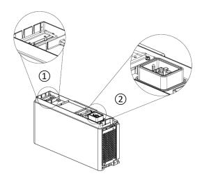
Figure 2-2-4 Structure diagram of battery module
