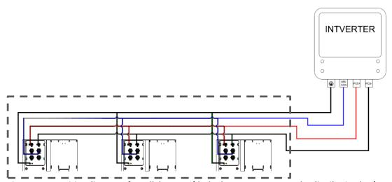
Figure 4-3-2a Wiring diagram of parallel system (dashed square represents the distribution box)
