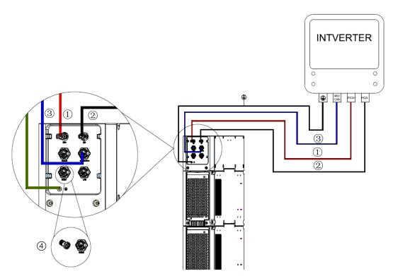
Figure 4-3-1 Wiring diagram of single machine system
