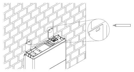
2 Drilling (for concrete or brick wall) and fixing the L-Bracket to the wall
