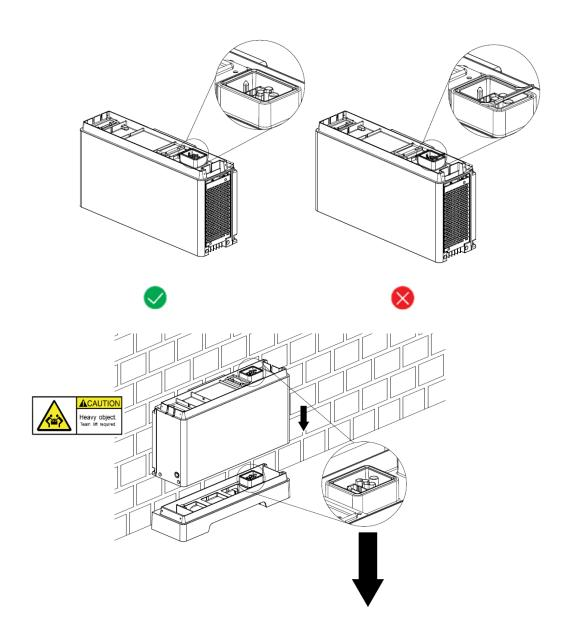
Unit weights 50kg (110.2lbs). Two or more people are necessary. Align the connector side first, then stack gently to avoid damaging the connector!
