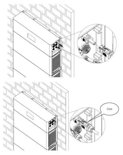
When pulling out the DC terminal, press the clips on both ends of the connector and then pull it out, as shown in the figure.
