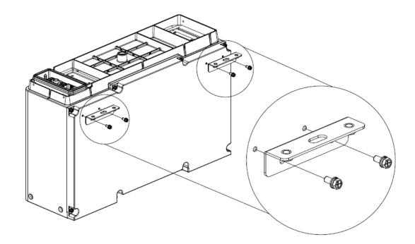
Refer to the following for the recommended the wall mounting assembly (angle bracket + L-bracket) installation:
