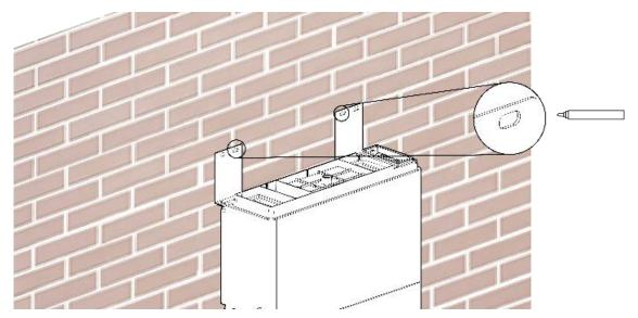
2 Drilling (for concrete or brick wall) and fixing the L-Bracket to the wall
