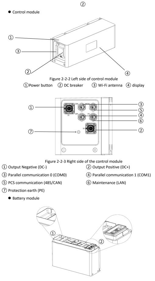
Figure 2-2-4 Structure diagram of battery module ① Handle ② Power/communication connector
