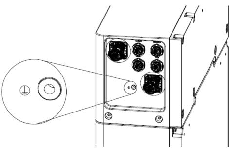
Figure 4-1-1 Schematic diagram of equipment grounding
