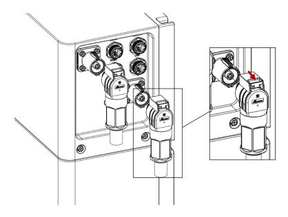
b. Lock the connector by pushing forwards the red/black buckle after insertion
