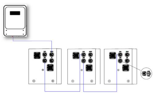
Figure 4-3-2b Communication wiring of multiple system
