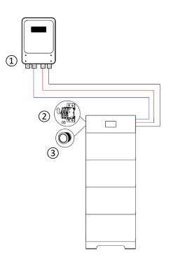
Note: Each cluster of battery systems in parallel system is powered on independently. When one cluster of batteries is powered on, close the circuit breakers of other clusters, and the other cluster of battery systems will be powered on automatically.
