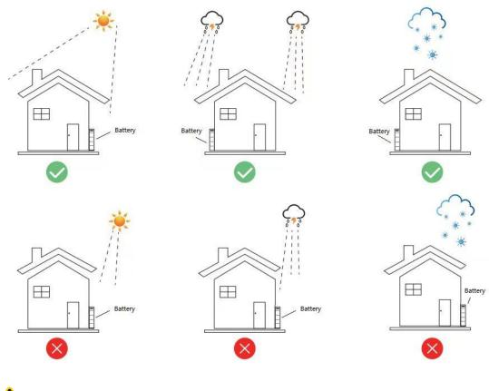
SunESS performance degrades when ambient temperature is below  $10^{\circ}C(50^{\circ}F)$  or above  $40^{\circ}C$
